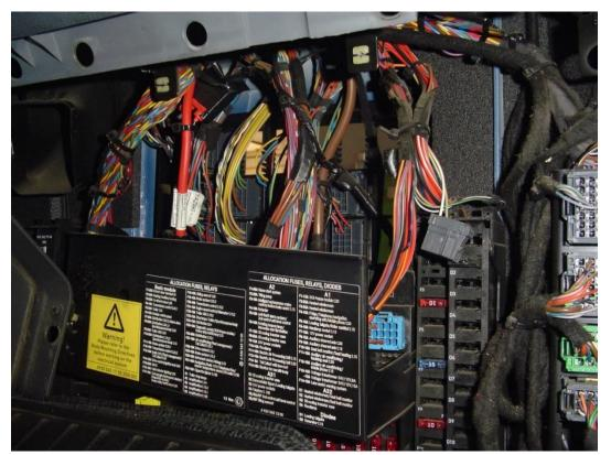
On this side mount device, one connector from the front of the are connecting, lead it through the hole, and the other connector put in the free place in the second row (cab-chassis connection box, used as a connector bracket).
