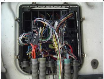
Disconnect the connector which is in sixth column of the machine left side (marked X6) and in the second line from the top:
