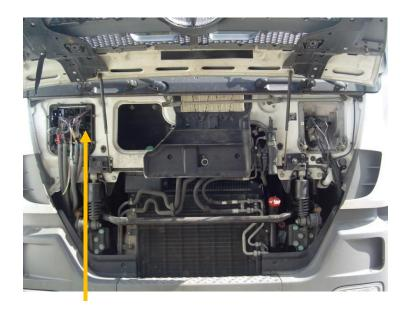
2 Open cab-chassis connection box (cable distribution panel) (indicated by arrow)
