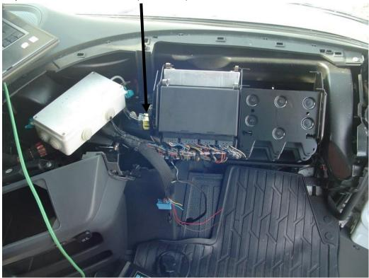
3 step. Solder cables to a CAN line according to below scheme N 1:
