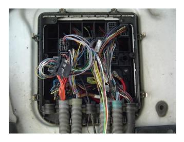
4 step. Disconnect the connector, which is in sixth column from the machine left side (marked X6) and in the second line from the top:
