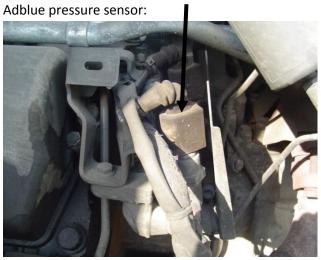
9 step. Block Adblue pump channels so that will stop Adblue liquid:
