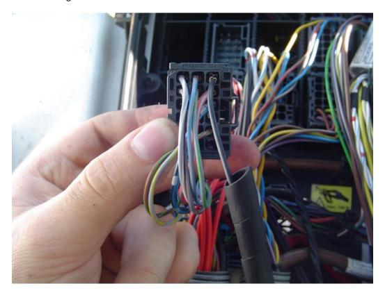
Pressure sensor cable can be founded under the cab on the engine near the start / stop switch:
