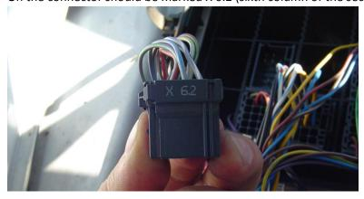
5 step. The gap are connected with cable connectors: one connector with connector socket, which left in the cab-chassis junction box from the top of the second row and the sixth column and the second connector put in free place in cab-chassis connections box. Connector should place like that the cables
