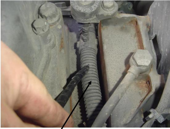
8 step. In this cable of wires we find a yellow wire with a purple ribbon, cut it and connect the cable which comming from the engine control unit (PLD) side. An advice. You can lead two wires and other wire connect to a pressure sensor side. Then, when you need to unplug, it will be enough just a short-
