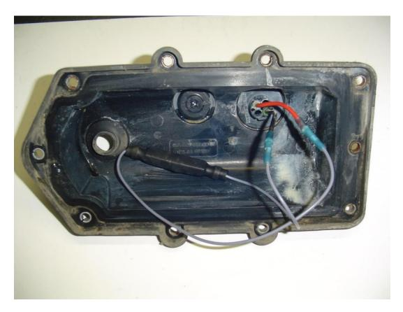
13 step. Insert the resistance of the pump inside the cap, so that it will protect against mechanical damage:
