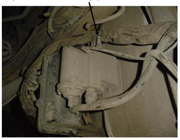
In the photo below are nozzles in which are built-in bolts, which blocks the channels:
