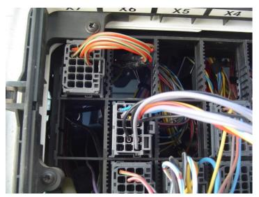
On the connector should be marked X 6.2 (sixth column of the second row):
