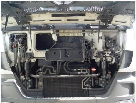
3 Step. Open cab-chassis connection box (cable distribution panel).
