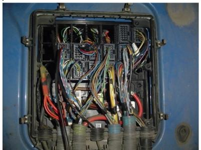
6 step. The device main module is installed in the cab inner side
