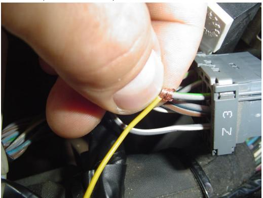
4 step. The white cable connected to the trimmed grey / green wire end, which goes into the SCR:
