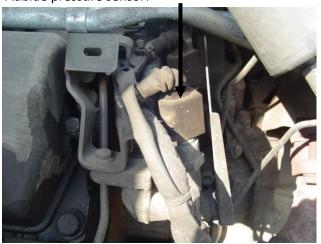
10 step. Block Adblue pump channels so that will stop Adblue liquid:
