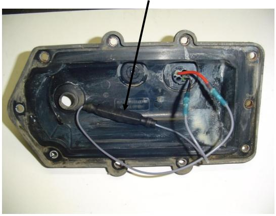
14 step. Insert the resistance of the pump inside the cap, so that it will protect against mechanical damage:
