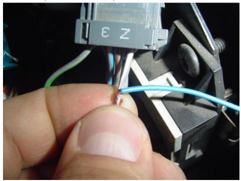
3 step. Yellow wire is connected to the trimmed grey / green wire end, which goes into the connector Z3 (3 contact in connector):
