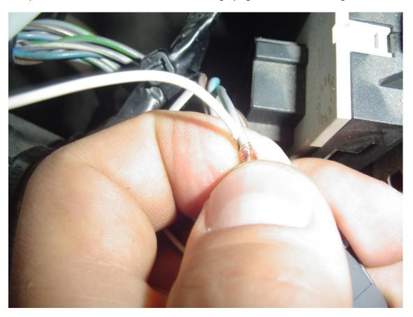
5 step. The black cable connected to the trimmed grey / white wire end, which goes into the SCR:
